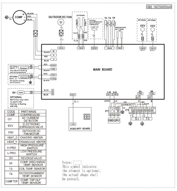
6.2 Wiring diagram of 1 drive 3 outdoor
