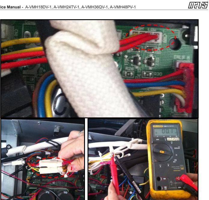
7.4.2.10 P3/PC 08 (Current overload protection)/ PC 44(Outdoor unit zero speed protection)/PC 46(Compressor speed has been out of control)/PC 49(Compressor overcurrent failure) diagnosis and solution.
