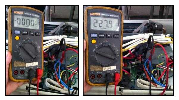
2 Turn off the power, use a digital tester to measure the resistance. The value should be  $1.8 \sim 2.5 \text{ K}\Omega$ .
