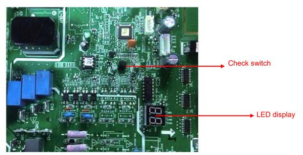
7.4.2.17 Communication malfunction between adapter board and outdoor main control board(ODU Ed)
